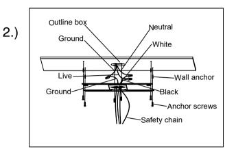
Step.2:Finish wiring(Black for Live,White for Neutral, and Green/Yellow Green for Ground.). Insert the head of safety chain into the bracket slot
