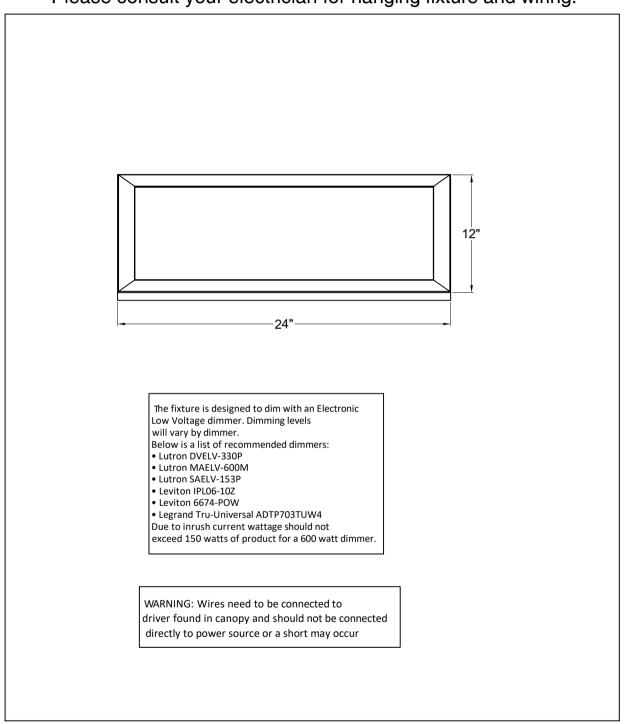
Bulbs(integrated): 120-277V Input and dimmable at 120V Integrated
